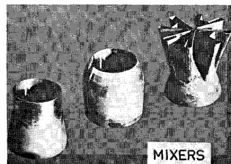
Fig. 8 Axial-flow mixer, injection mixer, and chute mixer.
